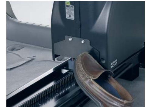
Safety plate obstruction sensor.
