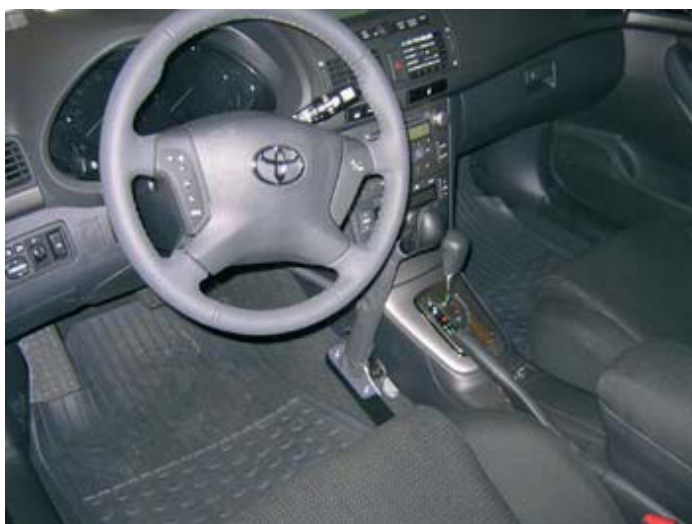
◀ The hand control Carospeed in a Toyota Camry
