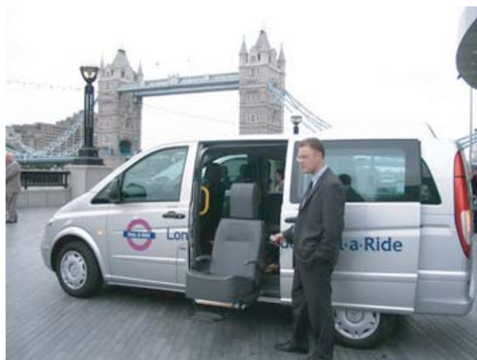
Autoadapt UK's Don Beattie tries the Turny Orbit in one of London Dial-A-Ride's new vehicles.
