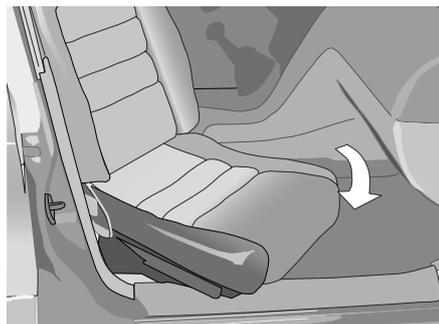
2. The seat rotates towards the outside as long as the left hand side button of the control is pressed down. At ultimate outer position the movement stops automatically.
