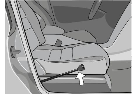
1. Adjust the seat lengthwise to optimize space for rotating the seat. Lift the release lever and start the rotating movement of the seat.
