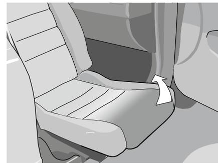
Adjust the seat if needed, to an optimal position for rotating it inside. The seat rotates towards the inside as long as the right hand side button of the control is pressed down. At ultimate inner position the movement stops automatically.
