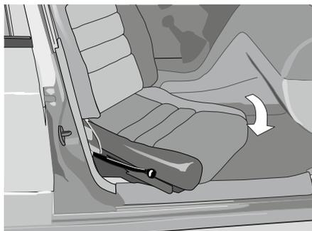
2. Let go of the release lever. Rotate the seat by holding on to the seat and not by pulling the lever. When the ultimate outer position is reached it locks automatically.
