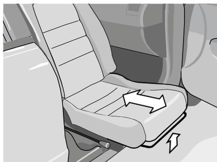
3. If needed, the seat can be adjusted further out by pulling the release for lengthwise adjustment.
