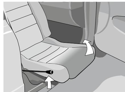
Adjust the seat if needed, to an optimal position for rotating it inside. Lift the release lever and start the rotating movement of the seat. Rotate by pushing the seat and let go of the release lever. Rotate the seat until it locks in its ultimate inner position!
