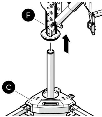
3 Remove the hoist (F) from the foot (C) by pulling it straight up.
