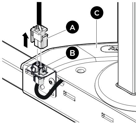
1 Remove the connector (A) from the socket (B) on the foot (C).
