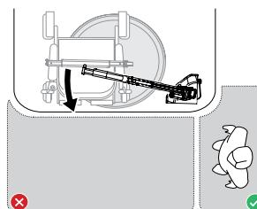
For safety when operating the hoist, make sure to stand in the operating safety zone and do not stand in the direction of the hoist's lifting arm.
